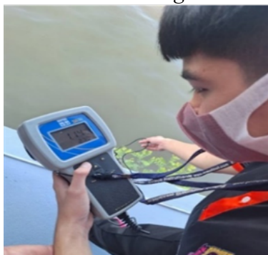
Students Measuring Dissolved Oxygen (Do) Levels in Canal Water
