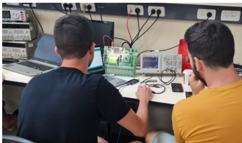
Figure 4. Pair of students validate signals by using equipment of a standard electronic laboratory
