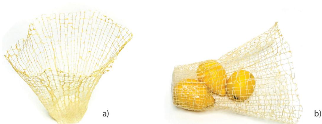
Figure 10. **Spider’s funnel-web bag with clementines dye:** a) empty bag, b) testing bag structure with approx. 0,5 kg of lemons, photo by authors
