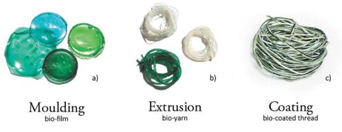
Figure 3. **Procedures Experiments** – a) alginate Bio-films; b) alginate Bio-yarns; c) bio-coated seaweed thread, from authors, photos by Luís Silva Campos
