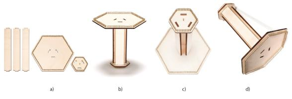
Figure 9. 3D loom boards and assembled views: a) disassembled boards,b) base view, c) top view, d) weaving seaweed-thread sample,from authors, photos by Luís Silva Campos
