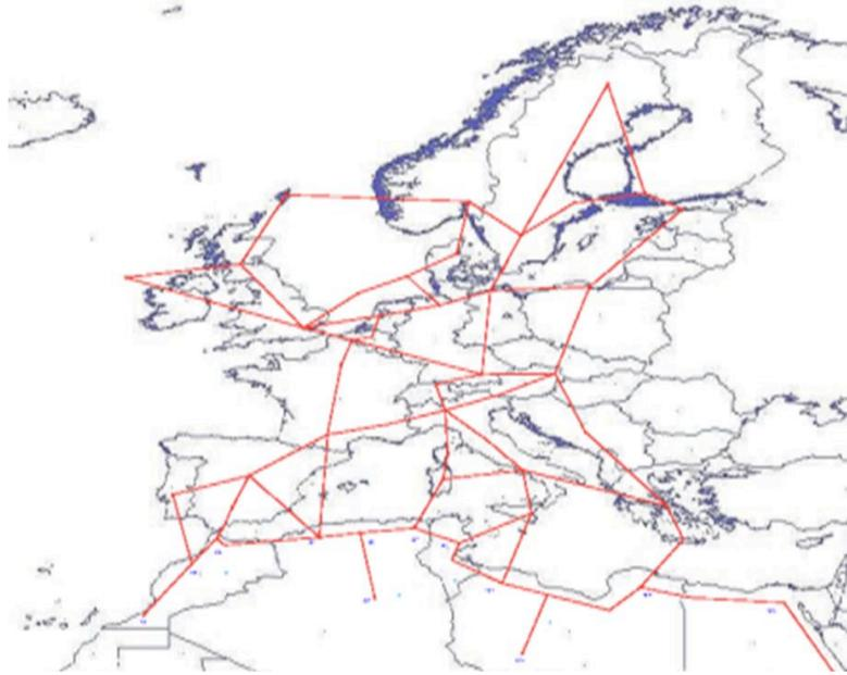
Figure 7. Pan-European-North African overlay HVDC transmission grid
