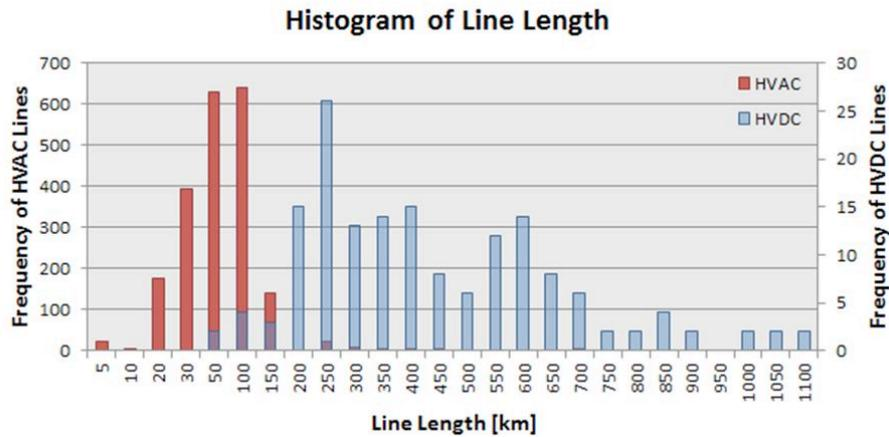
Figure 1. Frequency of transmission line length for HVAC and HVDC lines
