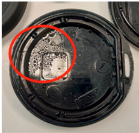
Figure 2: Water seepage (circled) in the MGA ‘watch’
