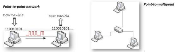
Figure 4: Point-to-point and point-to-multipoint network.
