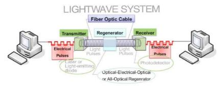
Figure 5: Point-to-point optical system.
