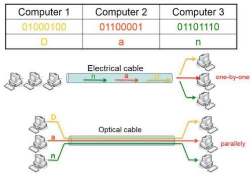
Figure 6: Wavelength Division Multiplexing technique.
