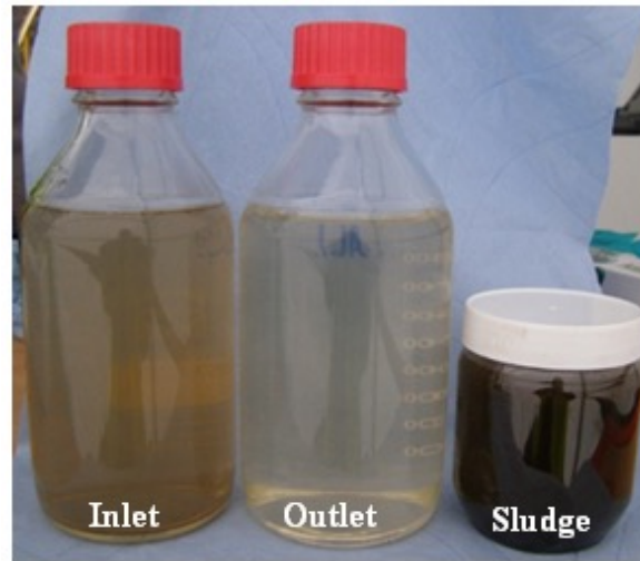
Figure 5: Inlet, outlet and sludge samples from Lab magnetic separator (2 m 3 /h)
