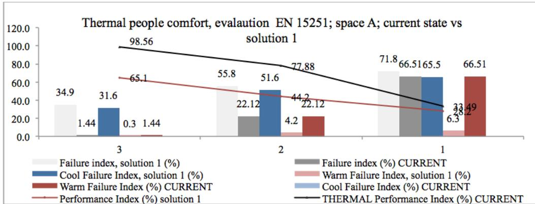
Graph 5.2.1; Thermal Performance Index (Pi) analysis EN 15251, space A current state versus solution 1
