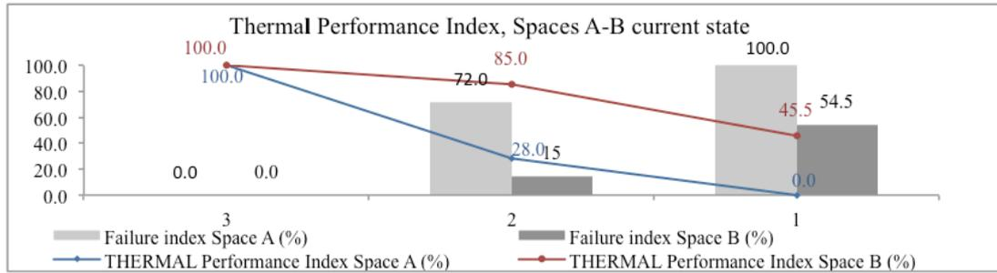
Graph 5.1.1; Thermal Performance Index (Pi) in space A and B; current state
