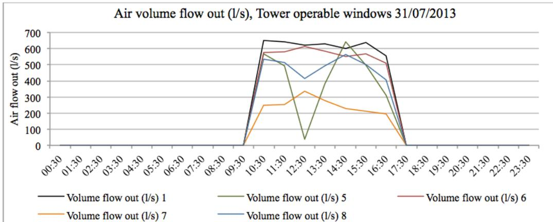
Graph 4.2. 3; Hourly air volume flow (l/s) through the outlet windows on the South tower
