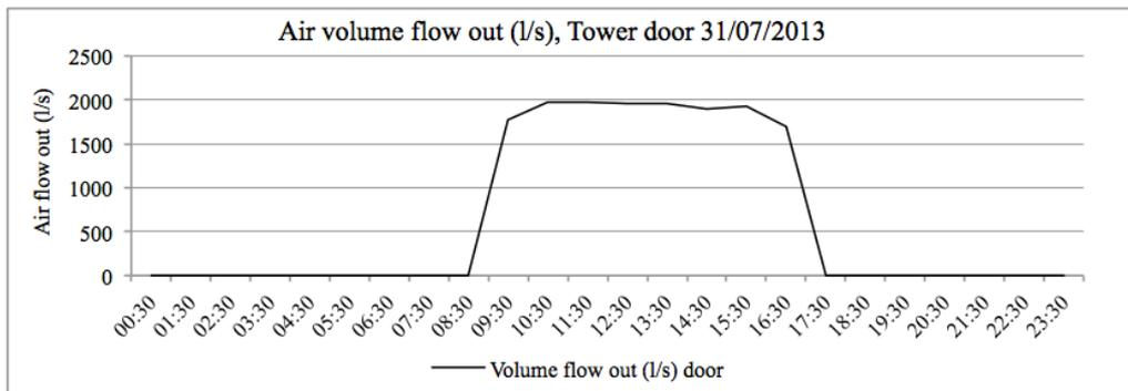
Graph 4.2. 4; Hourly air volume flow (l/s) through the outlet door on the South tower
