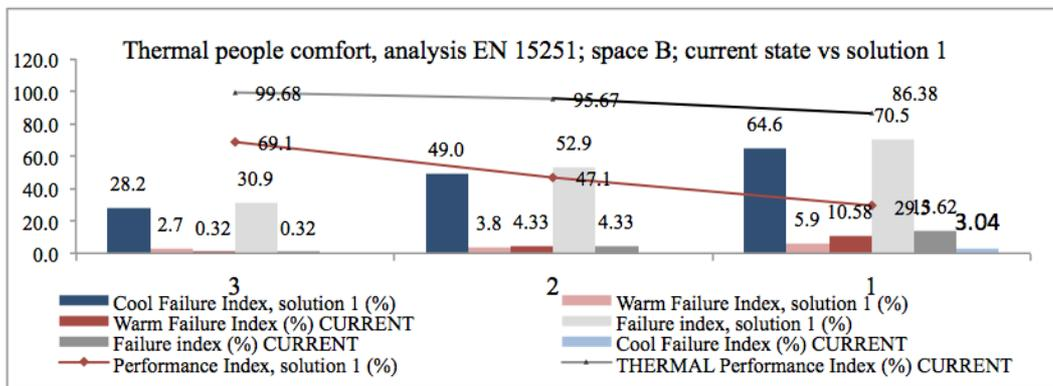
Graph 5.2.2; Thermal Performance Index (Pi) analysis EN 15251, space B current state versus solution 1
