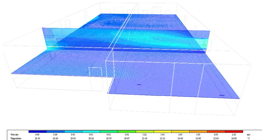
Image 5.2.1; Vertical and horizontal plans for air temperature and velocity tracking
