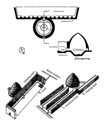
Fig 1. Left, Meibod Ice-pit in Yazd, this structure with a height of 15m is one of the tallest ice-pits in the city. Right, shading walls in the examples from Yazd [5].
