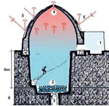
Fig 5. shows general section of the reservoir of a domed ice-pit, [5].
