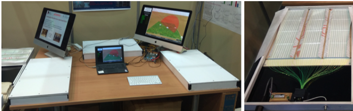
Figure 3: The \mu Cosmics telescope with 3 detection units (white boxes) and the interior of the detection unit (right).
