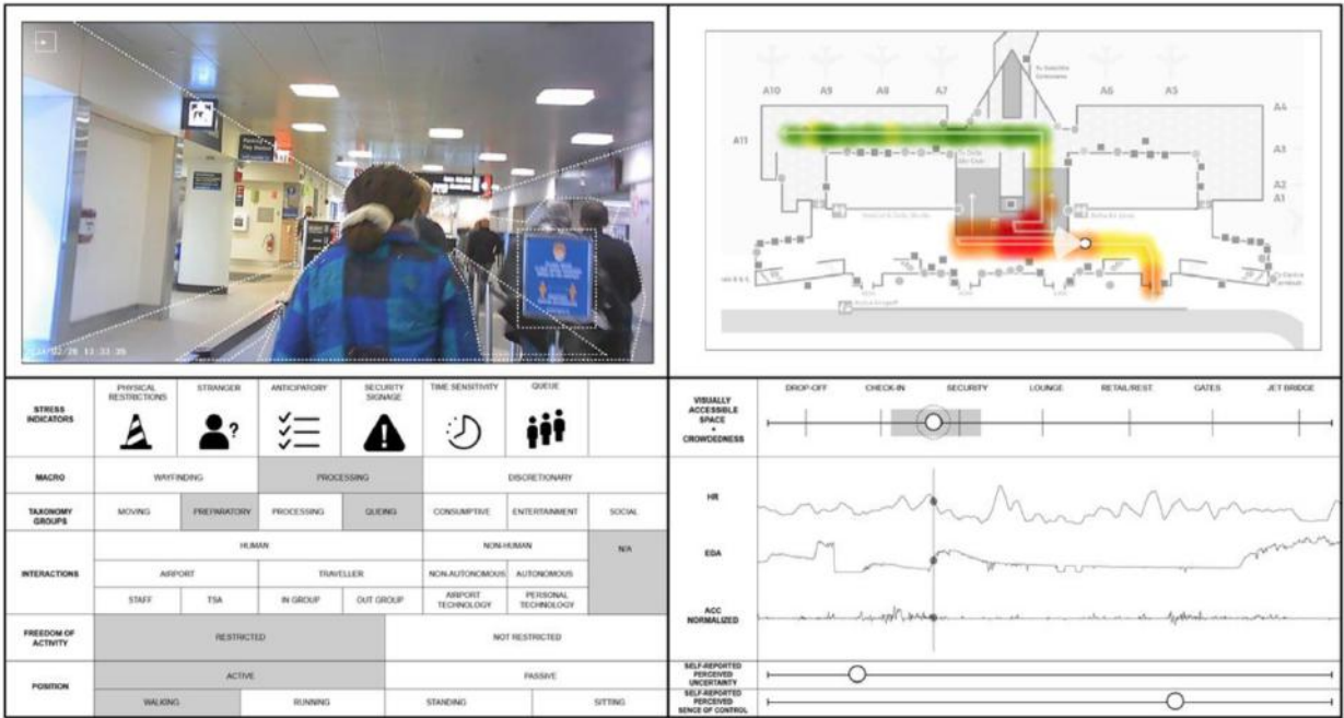
Figure 6. Draft dashboard visualizes biometric data, video, stress trigger activities and location within the airport.
