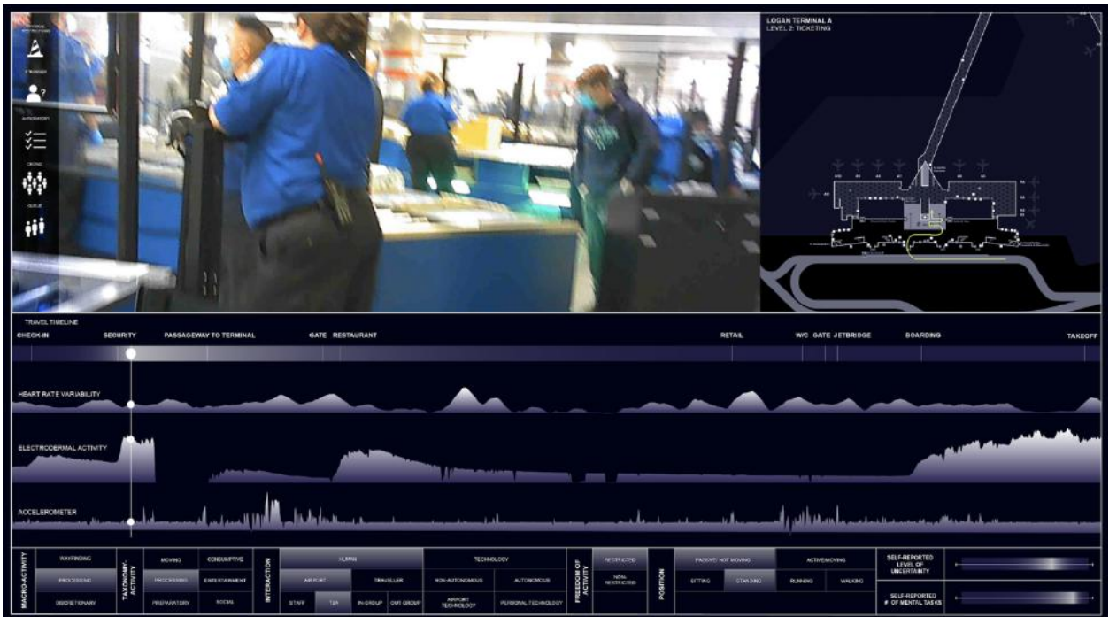
Figure 7. Finalized dashboard allows for cross-referencing of raw biometric data, video footage, spatial representation of stress, and stress trigger analysis.
