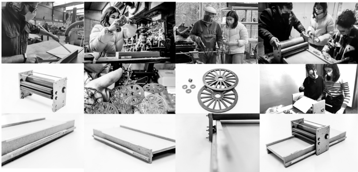
Figure 5: MDF boards and steel rods were cut by hand and holes were drilled with machines or by hand.
