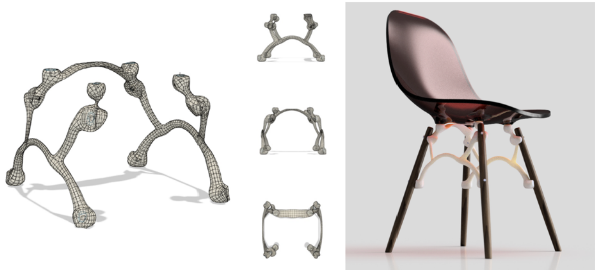
Figure 2. Digital prototype of replacement of steel yarn for chair Eames DSW (Vitra, 2018)
