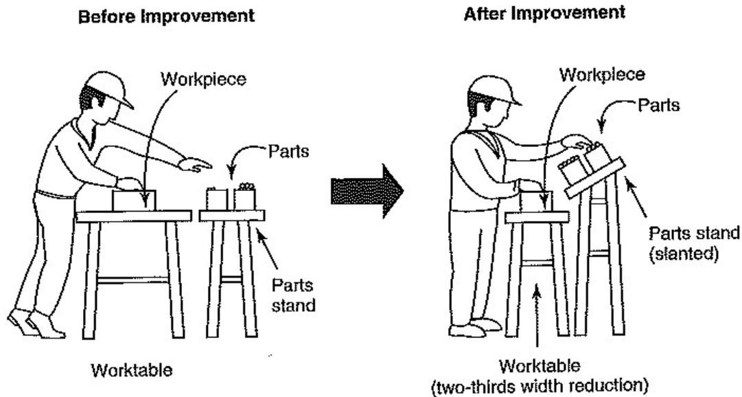
Figure 1: Example of excessive movement and its improvement
