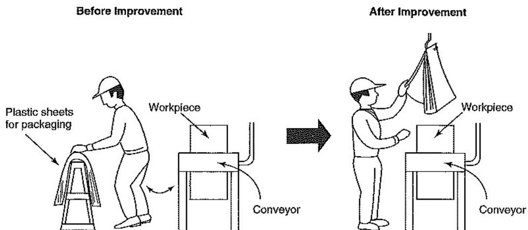
Figure 2: Example of excessive movement and its improvement
