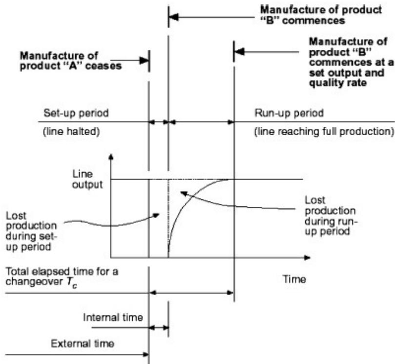
Figure 3: Setup operation period and the obtained output
