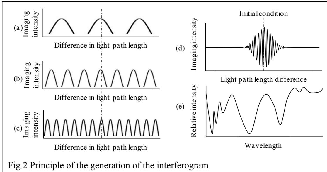
Fig.2 Principle of the generation of the interferogram.
