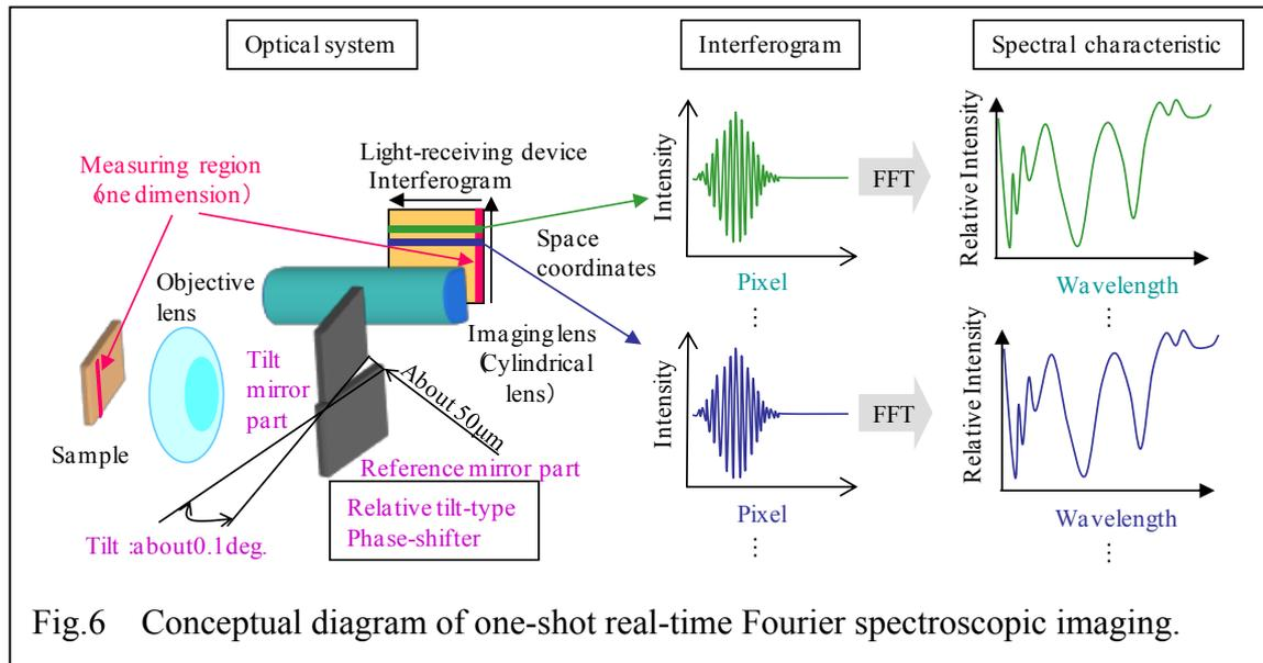
As shown in Fig.3, in each horizontal pixel-line, the interferograms are formed as the interference fringes by the spatial phase-shift. In other words, the spectroscopic characters are expressed as the periodical line-and-space fringes. And then, after these interferograms are calculated by Fourier transform algorithm, the spectral characteristics are obtained in each horizontal pixel-line. Thus, we can realize the one-dimensional Fourier spectroscopic measurement with one-shot imaging.
