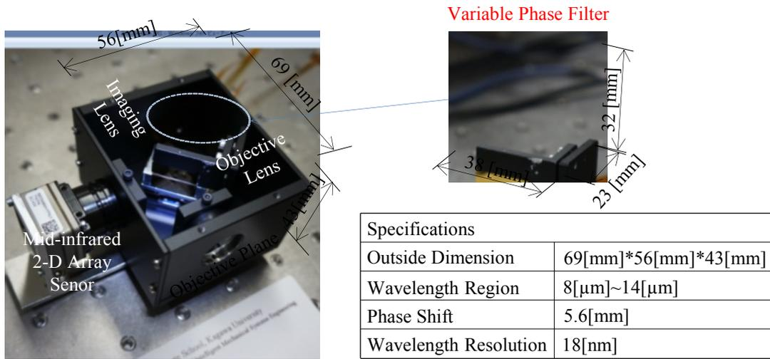
Fig. 3 The portable mid-infrared Fourier Spectrometer and specification
