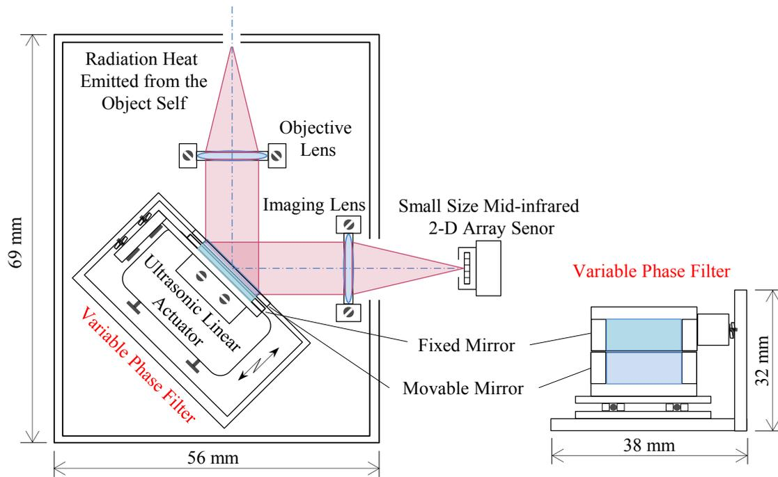
Figure 1. The schematic optical diagram of the imaging-type 2-dimensional Fourier spectroscopy
