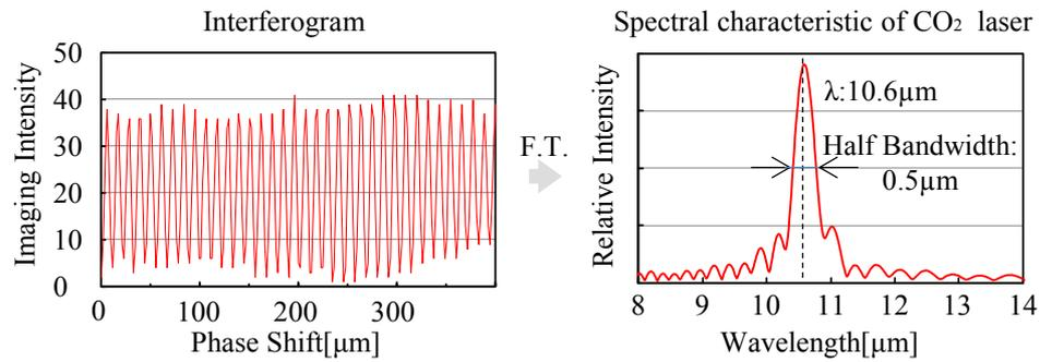
Fig. 4 Obtained line spectrum of CO<sub>2</sub> laser by portable mid-infrared Fourier spectroscopy apparatus
