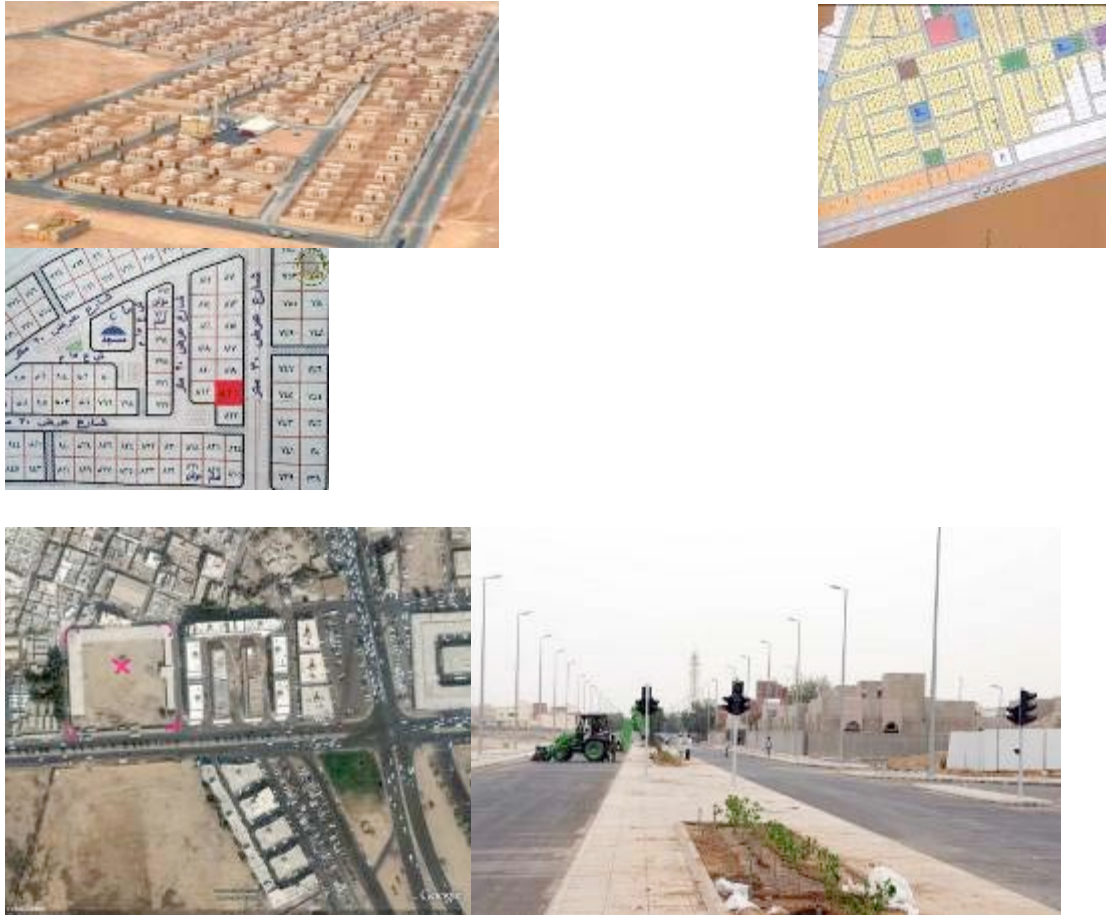
Figure 1: Example of some housing sites in Saudi Arabia: Almost no soft landscape was provided which will increase the use of energy for cooling or heating of dwelling units.
