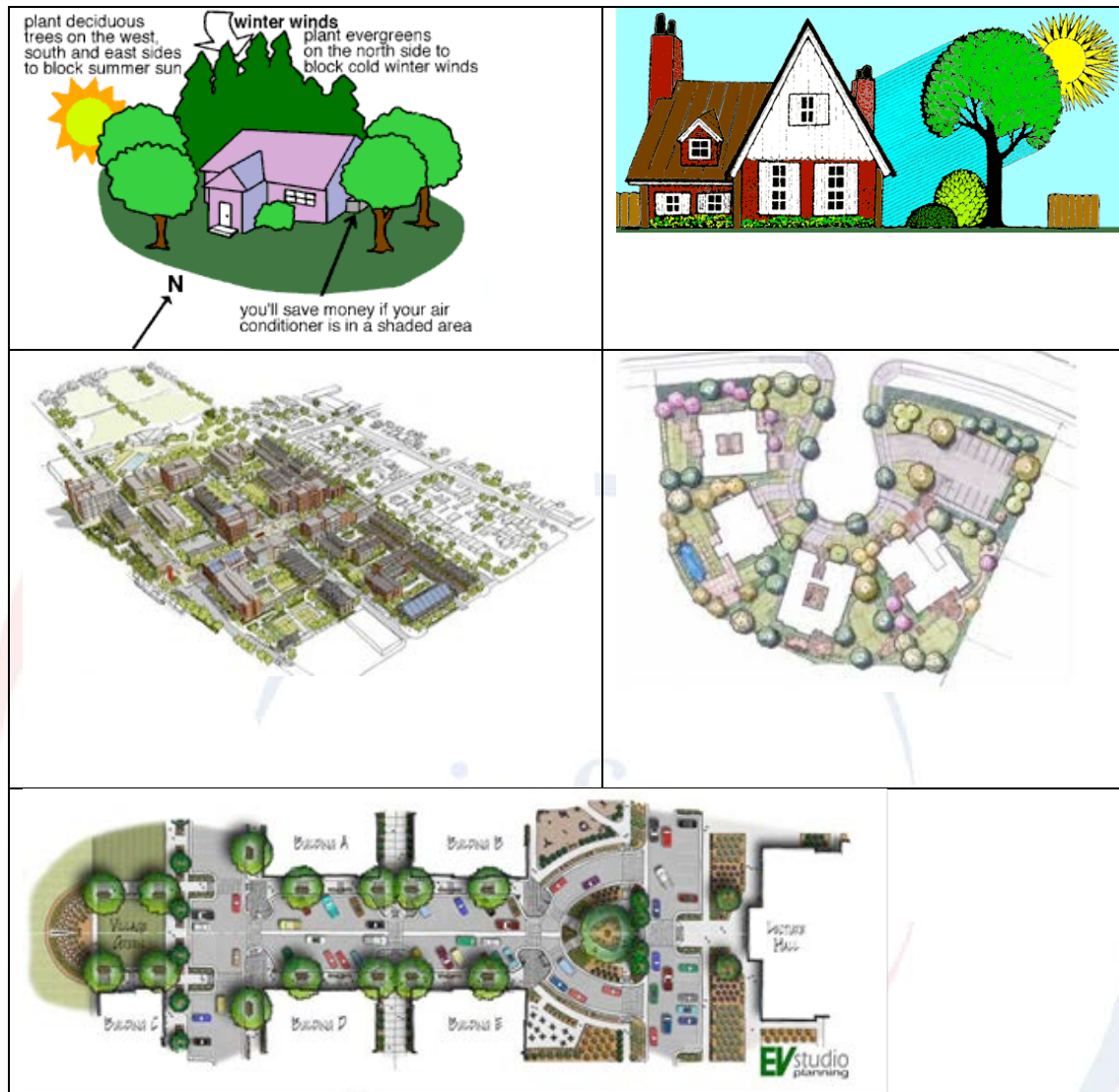
Figure 2: Soft landscape design can help save energy. Landscaping is an easy and economical way to increase the energy efficiency of the constructions, enhance the appearance and value of a property, and provide screening for privacy. Although outdoor landscape plants are pleasing in themselves, they can also play a large part in controlling energy use indoors. Therefore, it is important to consider the entire landscape plan in relation to energy conservation in all housing schemes.
