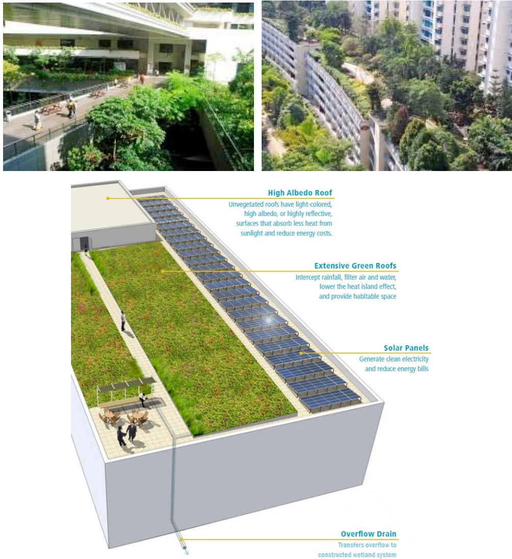
Figure 10: Green roof systems can be integrated with other green technologies. For example, green roofs and solar panels enhance each other's efficiency. Green roofs help cool ambient temperatures and allow solar panels to operate more effectively in hot weather. Solar panels shade vegetation and slow evaporation from green roofs, making it less likely that the vegetation will dry out.
