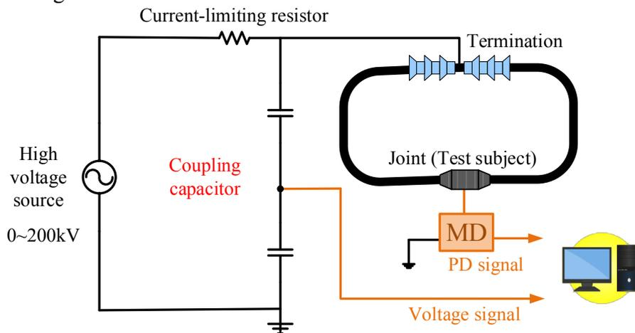
Figure 1: Cable joint experiment and partial discharges measurement.
