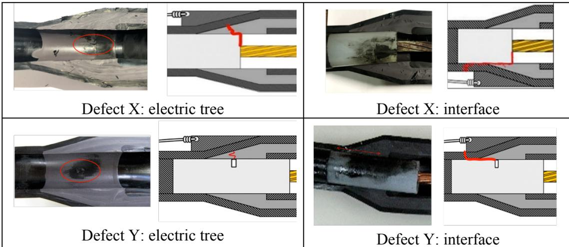
Figure 3: Anatomical photos and the schematic diagram of electric track
