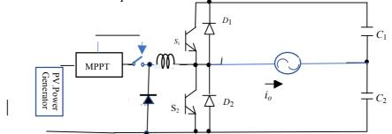
Fig.2. Power Conditioner with Compensation using Buck Converter.
