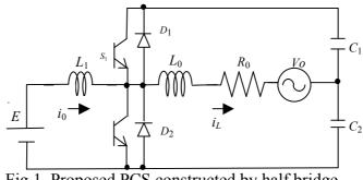
Fig.1. Proposed PCS constructed by half bridge.
