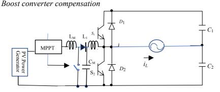
Fig.3. Power Conditioner with Compensation using Boost Converter.
