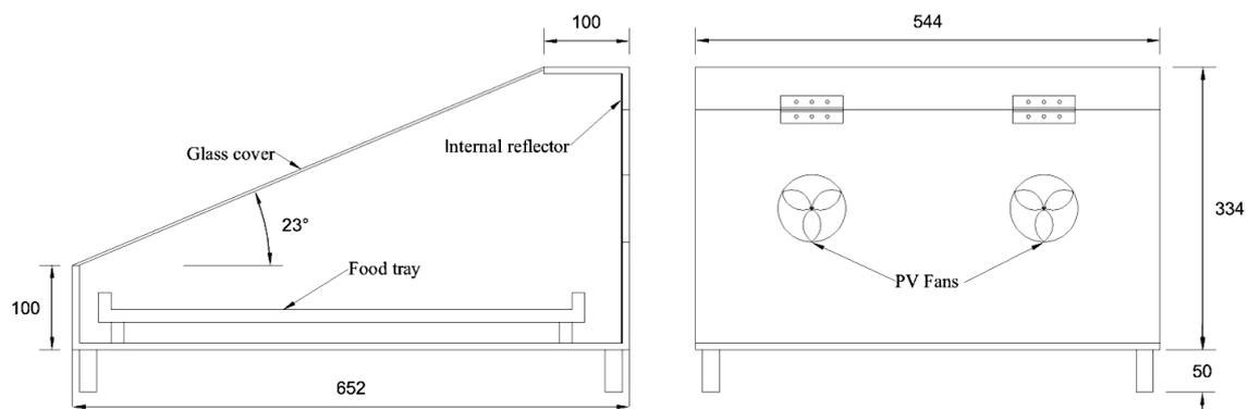
Figure 1: Schematic of proposed drying system
