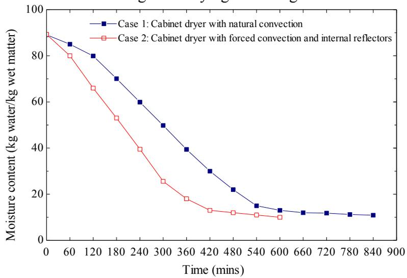
Figure 6: Variations of moisture content with time for a typical experimental run during solar drying of ginger
