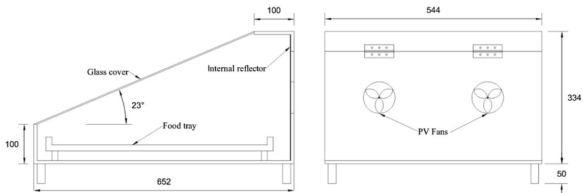
Figure 1: Schematic of proposed drying system
