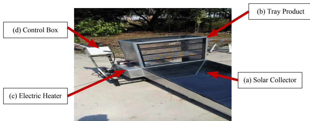
Figure 1. Solar dryer combine with electric coil
