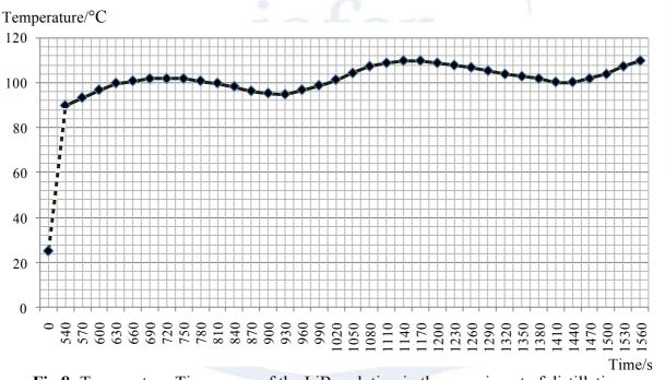
Fig.8: Temperature-Time curve of the LiBr solution in the experiment of distillation
