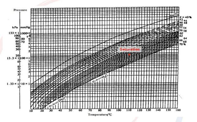
Fig.1: Saturated vapor pressure-Temperature-Concentration curve of LiBr solution [9]
