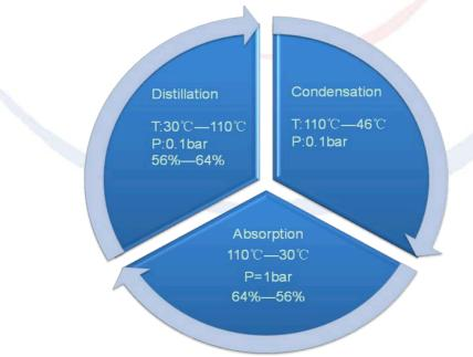
Fig.3: Cycle of the water collection system
