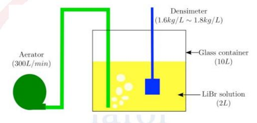
Fig.4: Equipment setup of experiments of absorption section
