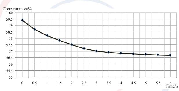
Fig.5: The concentration-time curve of LiBr solution in the Absorption cell
