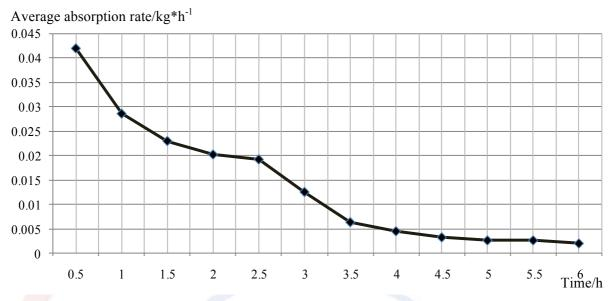
Fig.6: The absorption rate-time curve of LiBr solution in the Absorption cell
