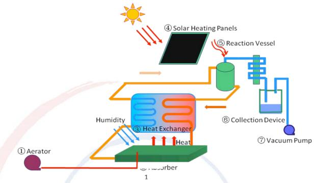
Fig.2: Sketch of the water collection system
