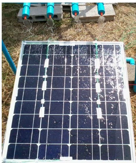
Fig. 2 The test PV with attached cooling system .
