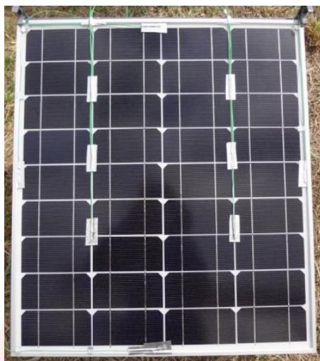
Fig. 1 The front surface of control PV with attached thermocouples.
