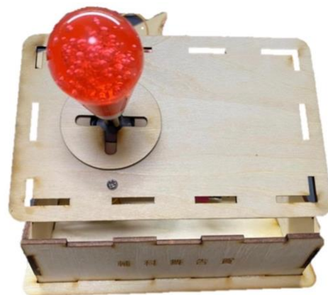
Fig. 2 Wooden Box Produced with Laser Cutting
