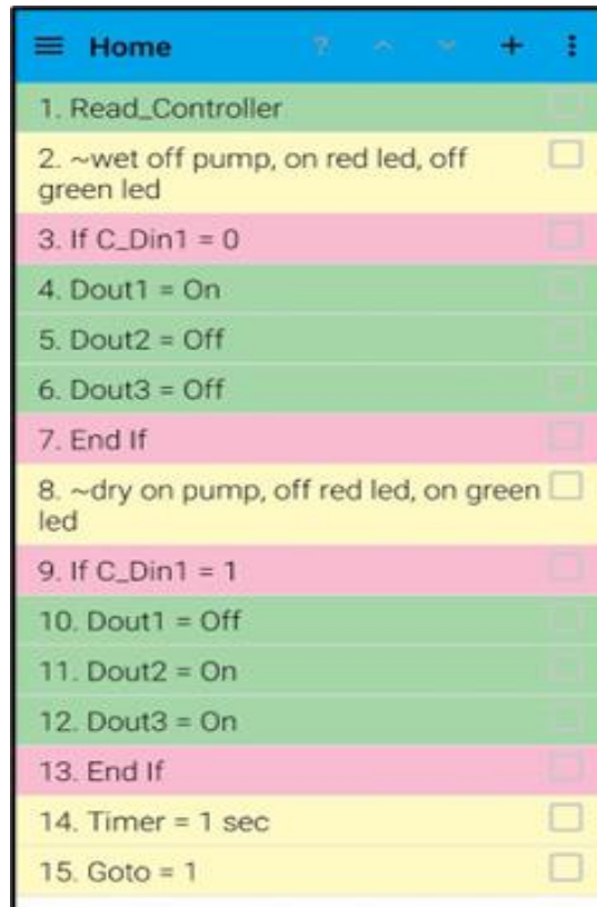
Figure 3: The Coding Command for Smart Irrigation System in Agricultural STEM-Based Project
