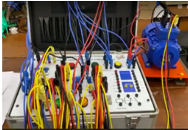
Figure 2: Manual operation of electric motor control circuit
