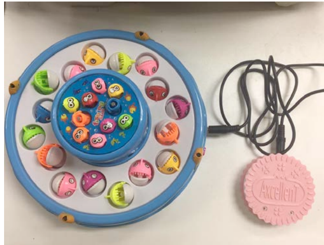
Fig. 5 A modified Toy and a Special Switch Connected with an Audio Cable
