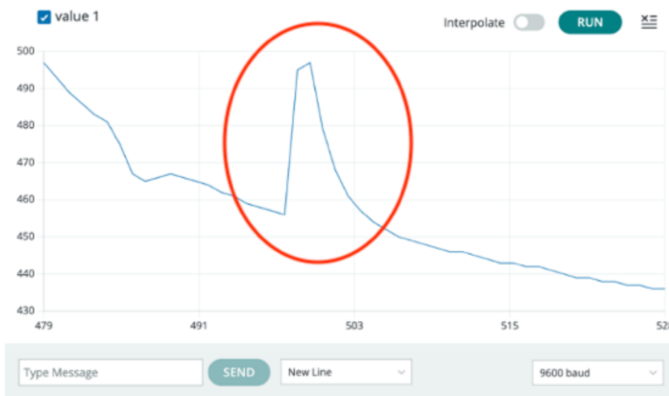
Figure 12: The waveform presented by Grove-GSR on Arduino
