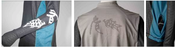
Figure 20 Laser cutting reflective material, mesh of Calligraphy and power bank pocket.
