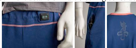
Figure 10 The electronic device in waist line and laser cutting mesh.
