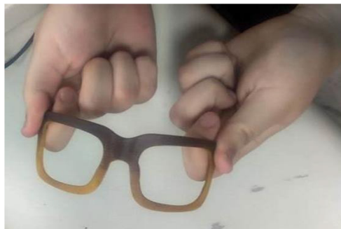
Figure 6: Elastic and bendable glass frame.
