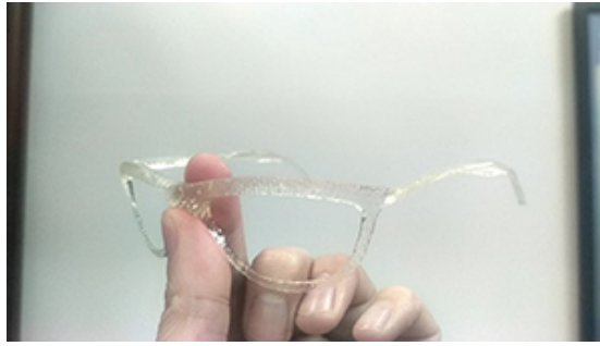
Figure 3: A glass frame printed by an UV laser 3D printer.
