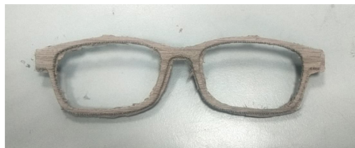
Figure 8: wood frame made by a CNC machine.
