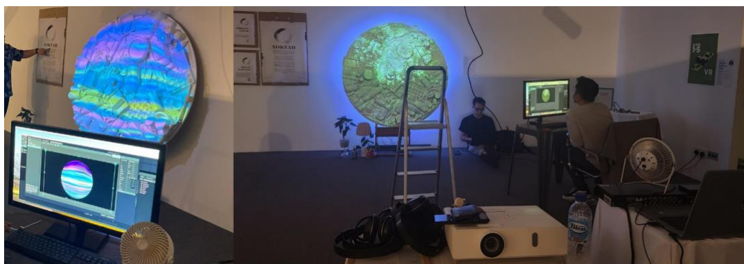
Figure 1: Calibrating Projection Mapping Onto an Uneven Surface
