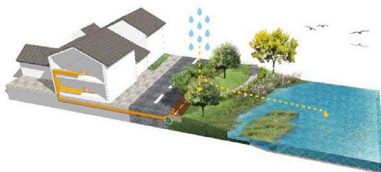
Figure 4: Rain water and sewage separation establishment in rural areas
