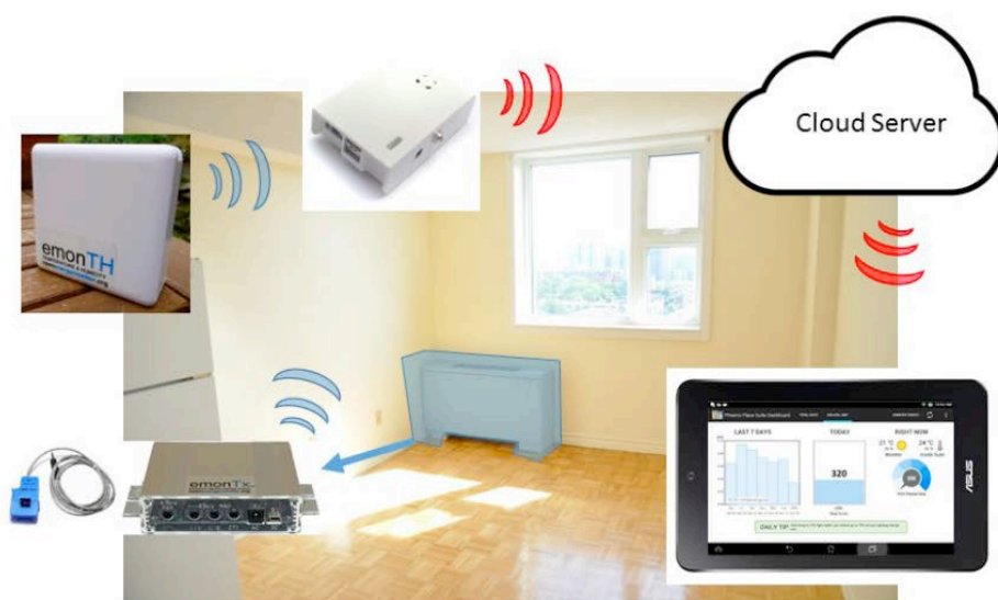
Figure 5: Rich-picture diagram of feedback hardware installed for each tenant. From bottom-left counterclockwise: emonTXv3 installed inside fan coil unit to measure power consumption and air temperature output, emonTH to sense ambient room temperature and humidity, a Raspberry pi gateway/hub, emonCMS cloud service, Android tablet with dashboard app. Additionally, but not pictured, were emonTXv3 units to measure suite-level power consumption.
