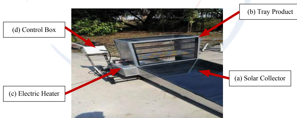
Figure 1. Solar dryer combine with electric coil
