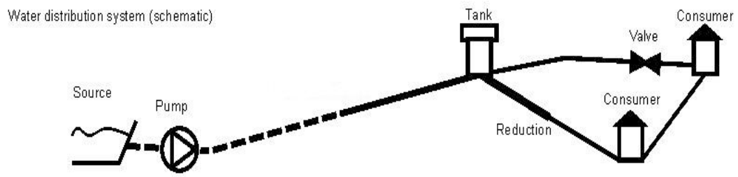
Figure 4. A Section of Water Distribution Network.
