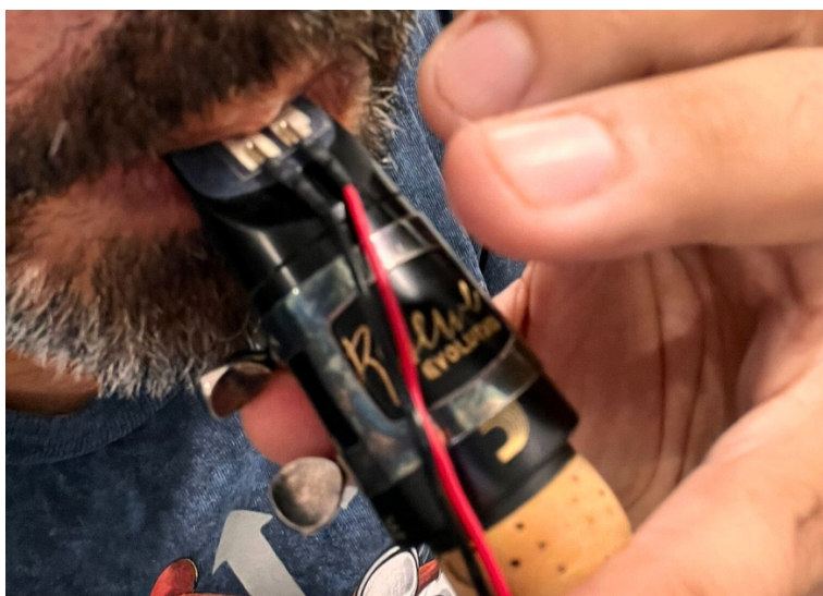
Figure 5. Sensor on the rubber of the mouthpiece.
