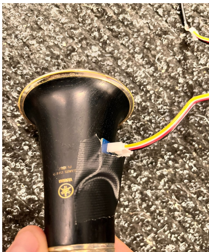
Figure 2. Switch placed over the bell.
