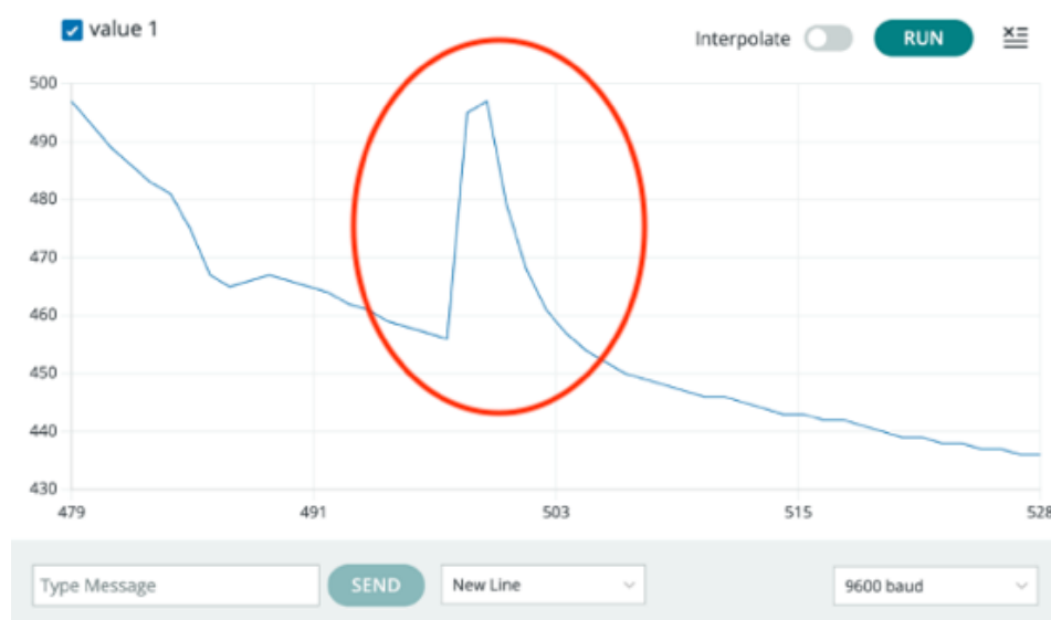
Figure 12: The waveform presented by Grove-GSR on Arduino
