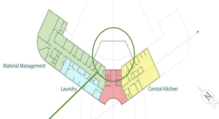
Figure 10. Basement floor plan; some change on the floorplan design and considering sunken courtyard bring natural lighting and natural ventilation for support departments (the picture retrieved from https://irandoostan.com/ir/iran-tour/tours-to-iran-civilization-persa-
