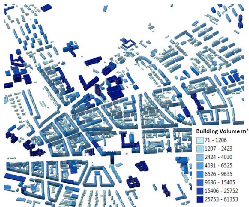
Figure 7: Calculation of building volume based on 3D city models. Source: Own depiction.
