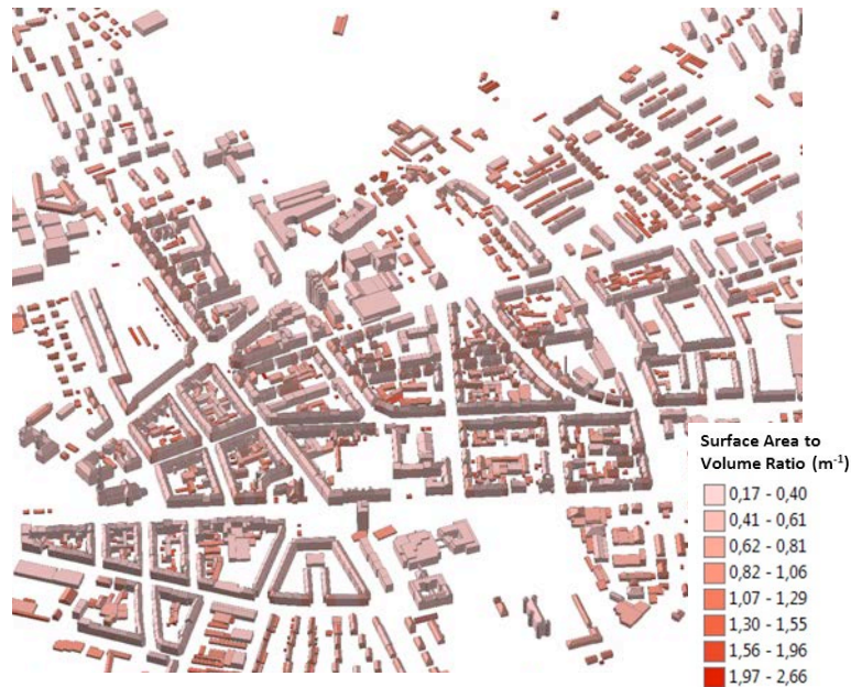
Figure 8: Calculation of building surface area to volume ratio. Source: Own depiction.
