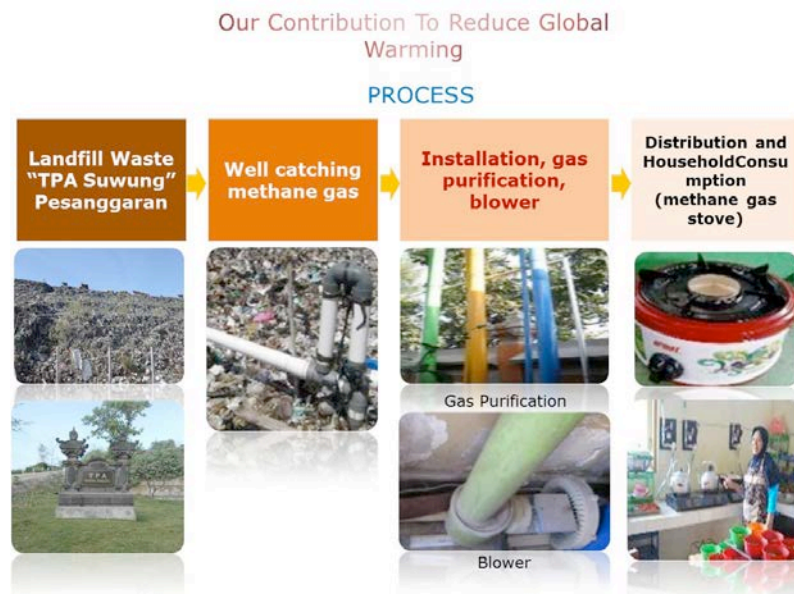
Figure 7. Schematic process of Methane Gas Utilization from TPA Suwung for Household Application [Mahendrayana, I.G.N., et al , 2017]
