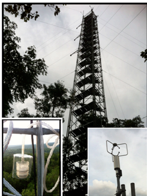
Figure 2: Aerosol and Black Carbon collectors on a 36 m- high tower at SBR
