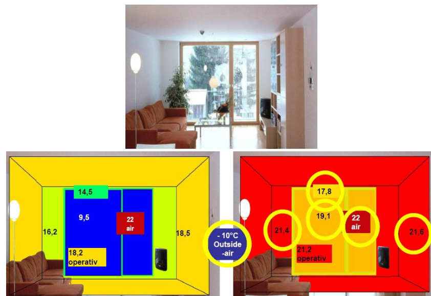
Fig. 1 Difference on thermal comfort between standard house and passive house
