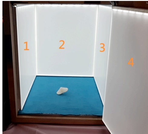
Figure 3: Four-sided LED lightening boarded recognition box
