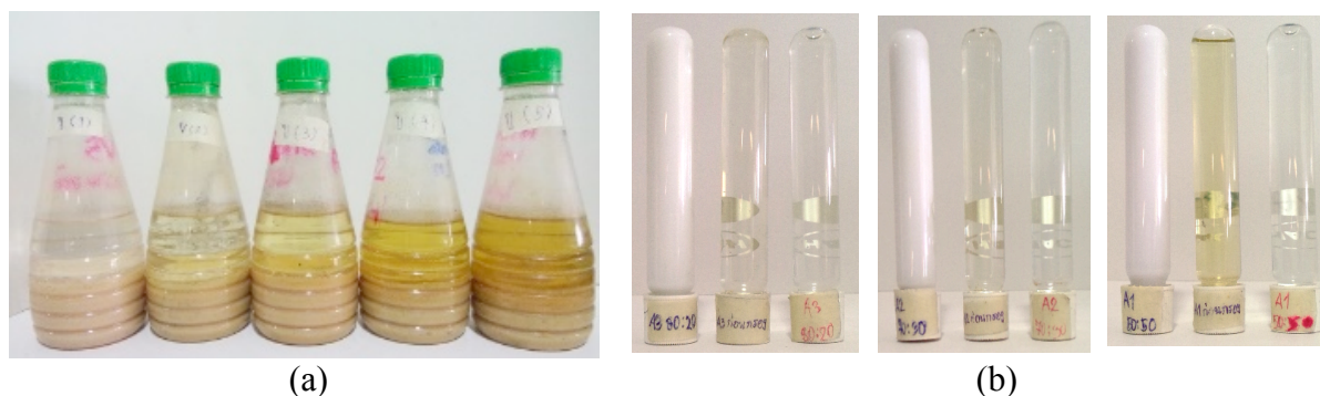
Figure 3: (a) Color of treated water after coagulation with different coagulant dose (b) Color of effluent, treated water after coagulation/filtering, and after adsorption with GAC
