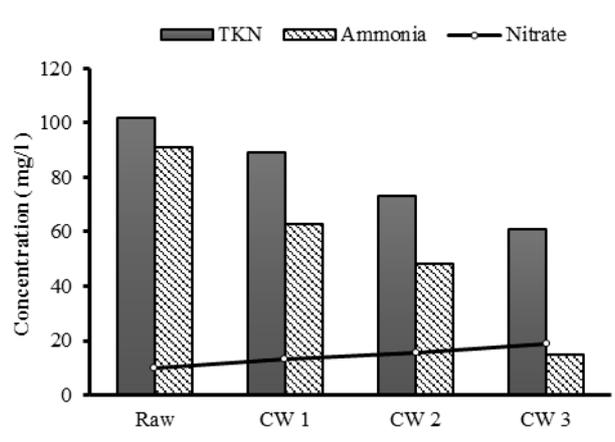
Figure 5: TKN, ammonia, and nitrates for influent and each reactor effluent.
