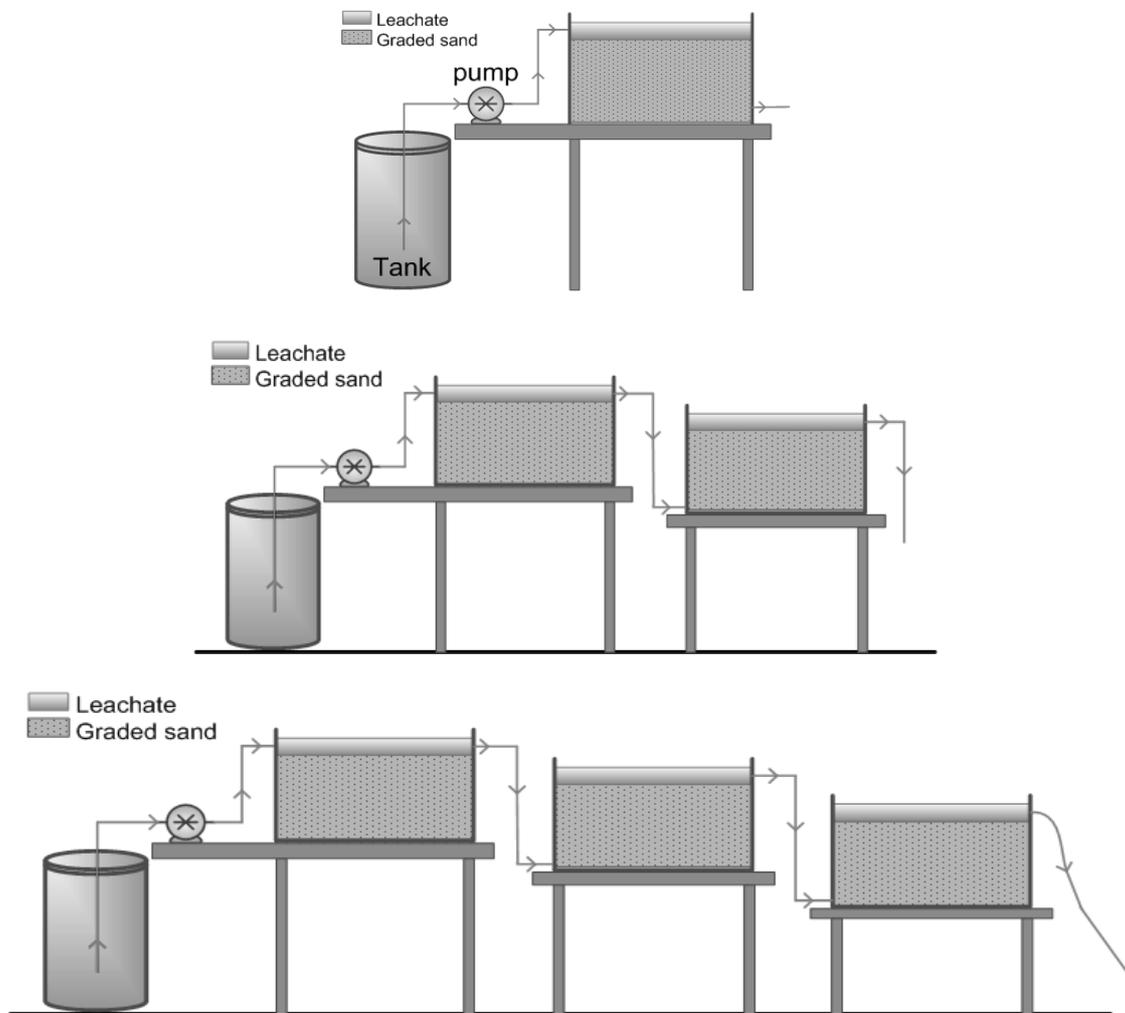
Figure 1: Schematic diagram for the three non-vegetated constructed wetland with graded sand bed systems.
