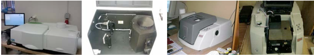
Figure 2 (a) UV/VIS/NIR Spectrophotometer Perkin Elmer Lambda 1050 with 150 mm Spectralon integrating spheres; (b) FT-IR infrared spectrometer Nicolet 380 and integrated sphere Mid-IR ™ IntegratIR
