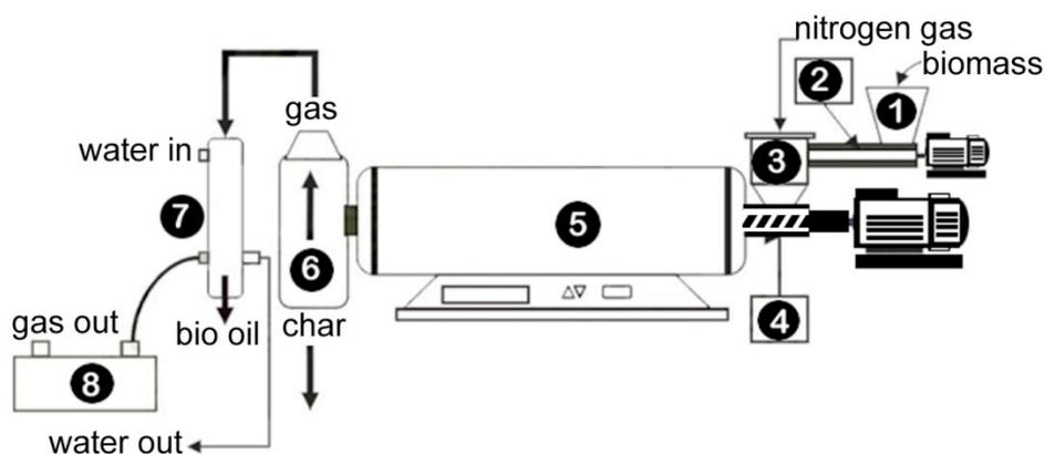
Figure 1: Schematic diagram for the continuous pyrolyser
