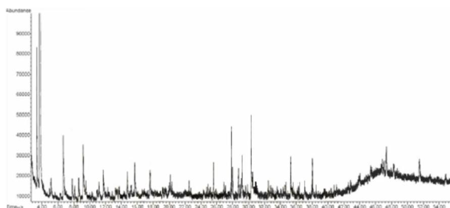
Figure 5: GC-MS Chromatograph on tar fraction
