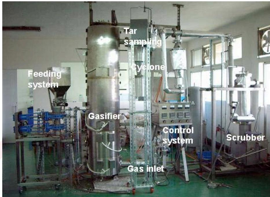
Figure 11 Pilot-scale gasifier
