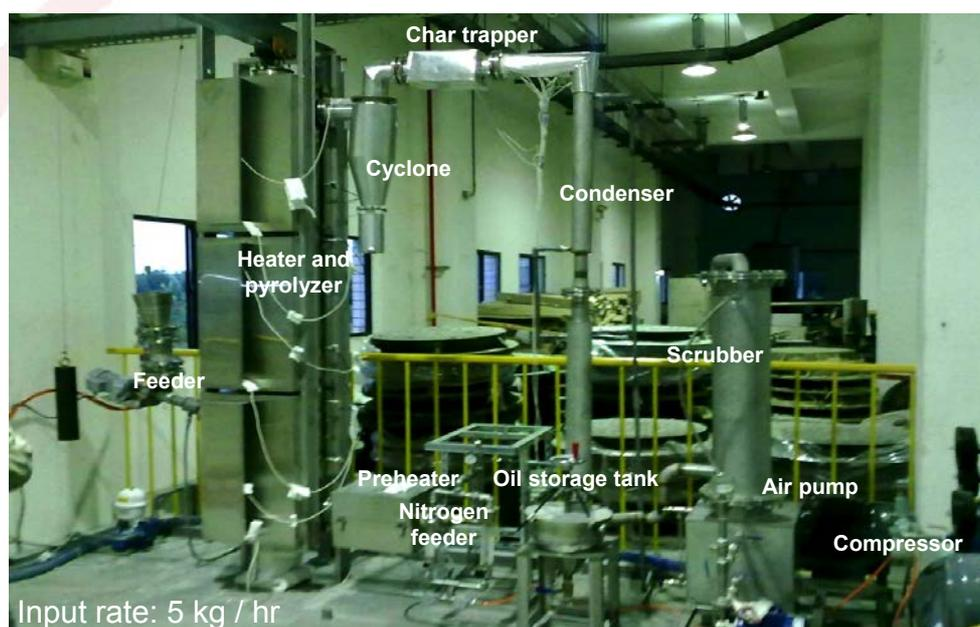
Figure 10 Pilot-scale pyrolyzer
