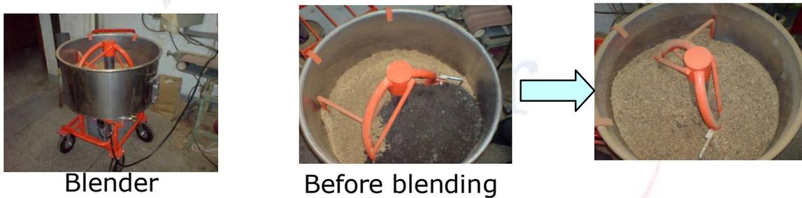
Figure 8 The blending of sludge and woody chips (sugi)
