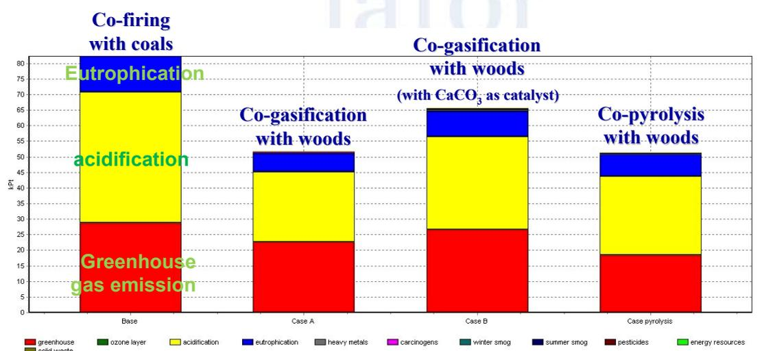
Figure 13 The comparison of four steam producing projects using Eco-indicator 95
