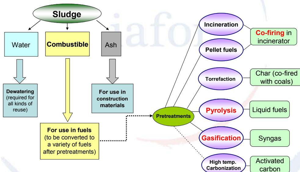
Figure 3 The possible energy application of sludge
