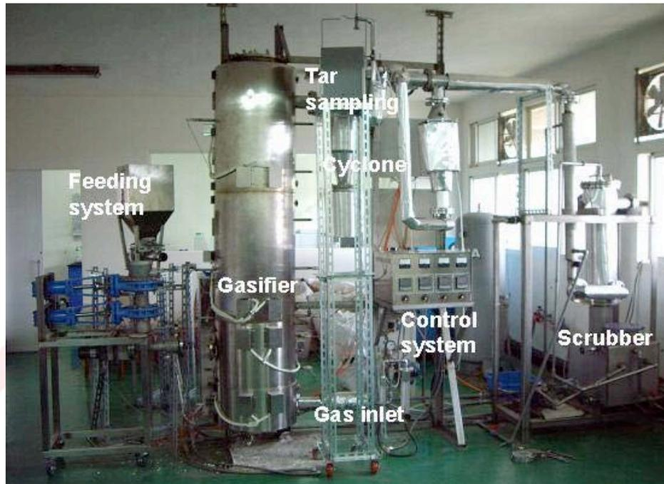
Figure 11 Pilot-scale gasifier
