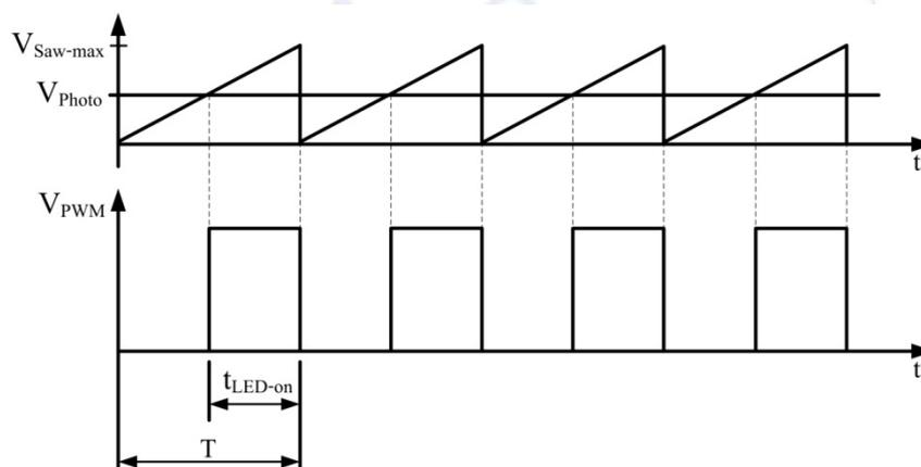
Figure 2. Showing the diagram of pulse width modulation signal.
