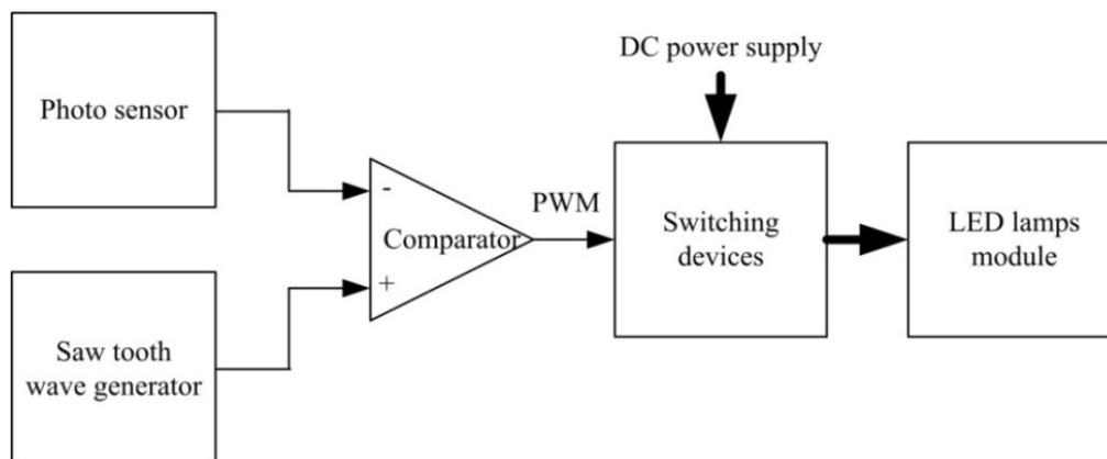
Figure 1. Block diagram of a lighting controller for LED lamps cooperated with daylighting.
