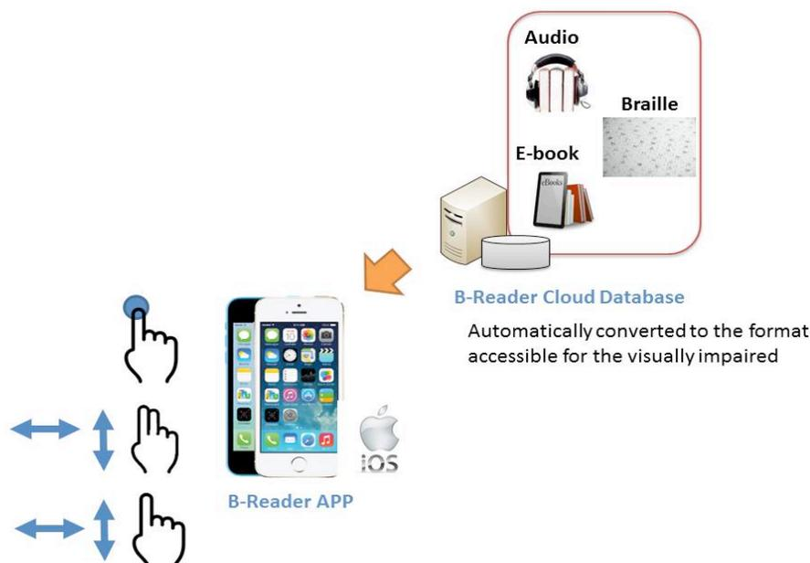
Figure 1: The architecture of the B-Reader system.
