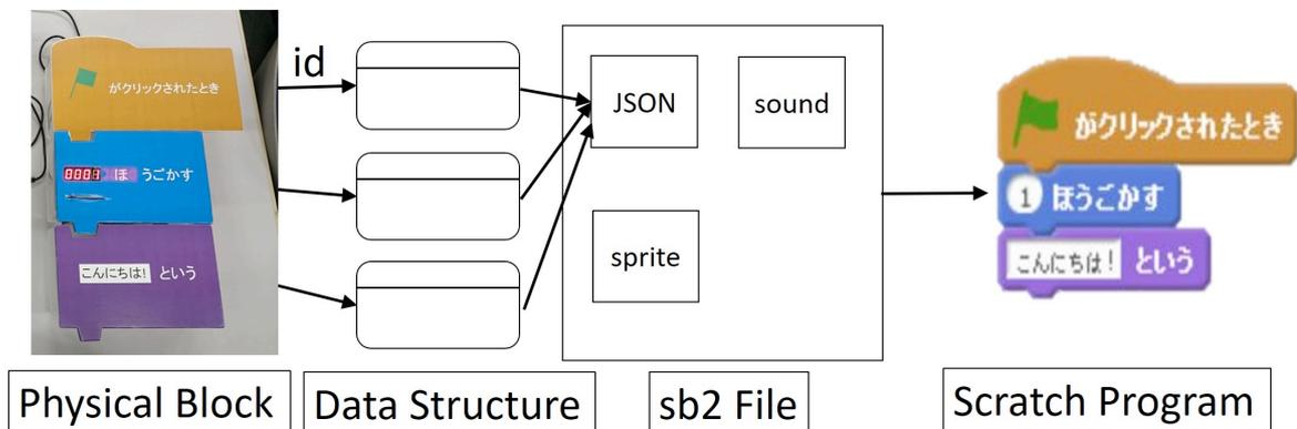
Figure 6: Construct a Scratch Program
