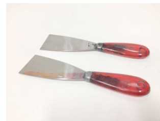
Figure 25: Ink knife, used for scraping the ink on the roller
