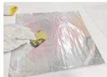
Figure 18: Sanding with Sandpaper to Create Rough Surface
