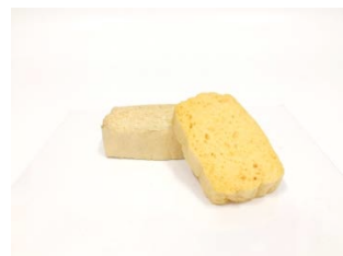
Figure 33: Cellulose sponge, used for damping the block to remain moistened at all times.
