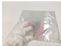
Figure 17: Placing Aluminum Foil Neatly onto Acrylic Sheet
